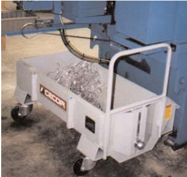
DB-L43-4P stands 15-1/2 inches tall and easily fits under machine tool discharge.
